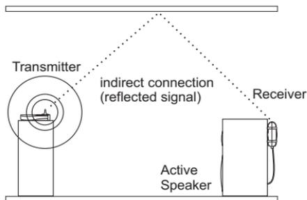
**Example 2:** Receiver mounted vertically behind a speaker
