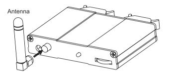
Turn the cap clockwise to fasten the antenna
